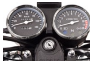
Large, clear speedo, tachometer and gear-position indicator
